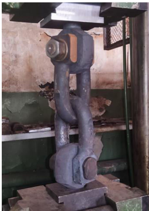
Рис. 8. – Installed mounting blocks on the UMM-100 machine
