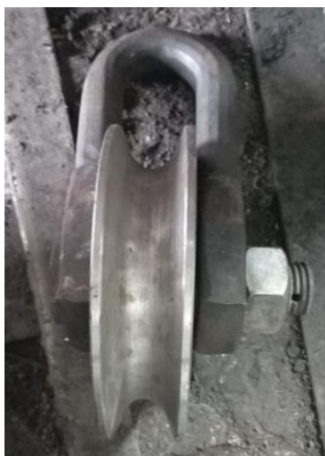
Fig. 1. - General view of the operating mounting block
