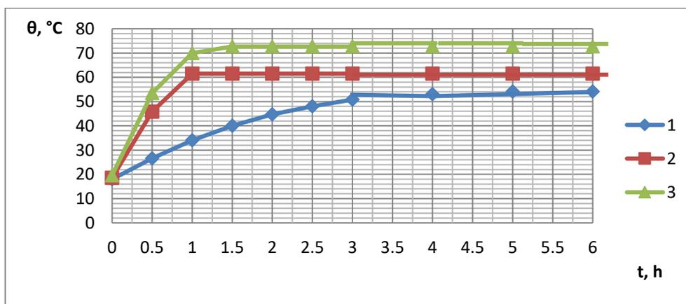
a) 1, 2 and 3 are curves of dependence of the water heating temperature at the diameter of the active ejector nozzle of 25 mm on the heating time at the volume of heated water of 70 dm<sup>3</sup> (1), 50 dm<sup>3</sup> (2) and 30 (3) dm<sup>3</sup>;
