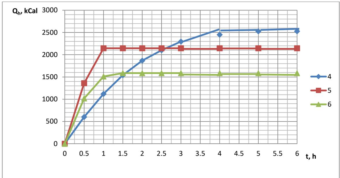
b) 4, 5 and 6 are curves of dependence of the heat obtained when heating water at an ejector of 25 mm on the heating time at a volume of heated water of 70 dm<sup>3</sup> (4), 50 dm<sup>3</sup> (5) and 30 (6) dm<sup>3</sup>
