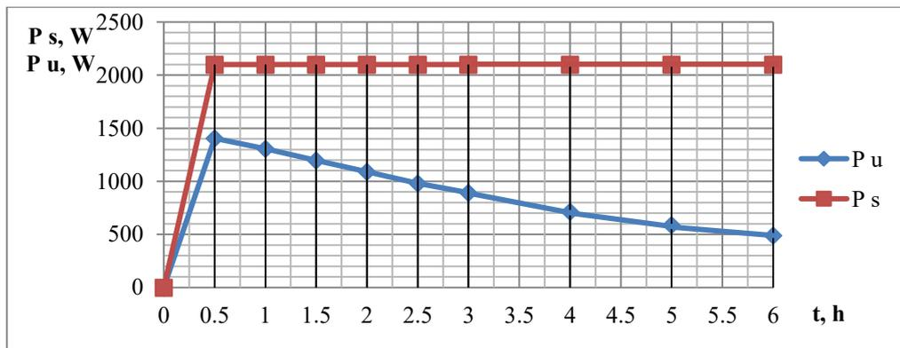
a) — curves of the dependence of the useful thermal power and the expended one with a diameter of the active nozzle of the ejector of 25 mm on the heating time with a volume of heated water of 70 dm<sup>3</sup>
