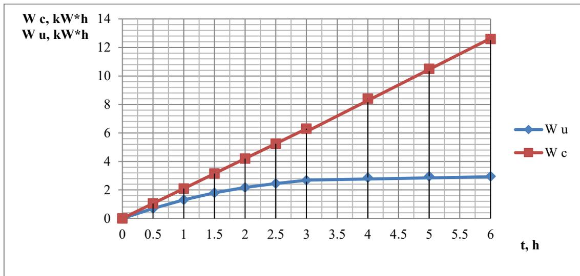
b) — curves of the dependence of the useful thermal energy and the spent at the ejector of 25 mm on the heating time at a volume of heated water of 70 dm<sup>3</sup>.
