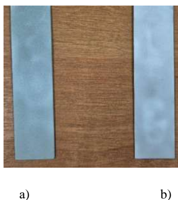
Fig.1. – Samples with gas-dynamic coating: a) CRO; b) NiAlSiCr
