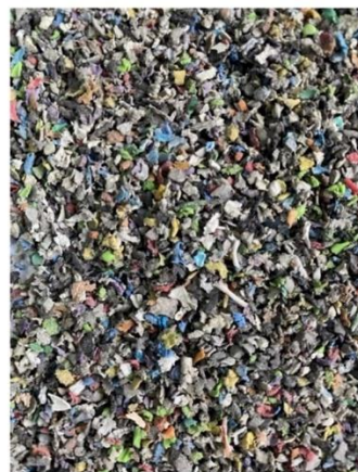
Fig. 2. – Plastic granulate constituting the insulation of electrical wiring in automobiles: a) After the shredding process with a 1.5 mm screen; b) After the shredding process with a 1 mm screen
