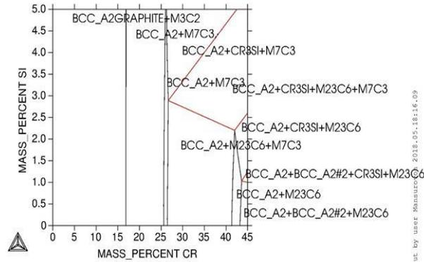
Fig. 5. Phase diagram of Fe-2.6C-Cr-Si, T=200 °C
