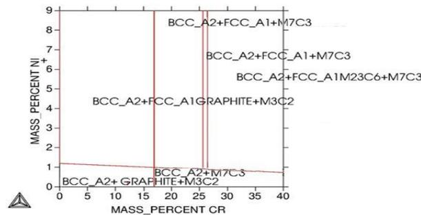
Fig. 3. Phase diagram of Fe-2.6C-Cr-Ni, T=200 °C
