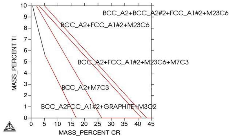
Fig. 6. Phase diagram of Fe-2.6C-Cr-Ti, T=200 °C
