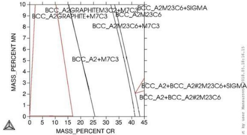
Fig. 4. Phase diagram of Fe-2.6C-Cr-Mn, T=200 °C
