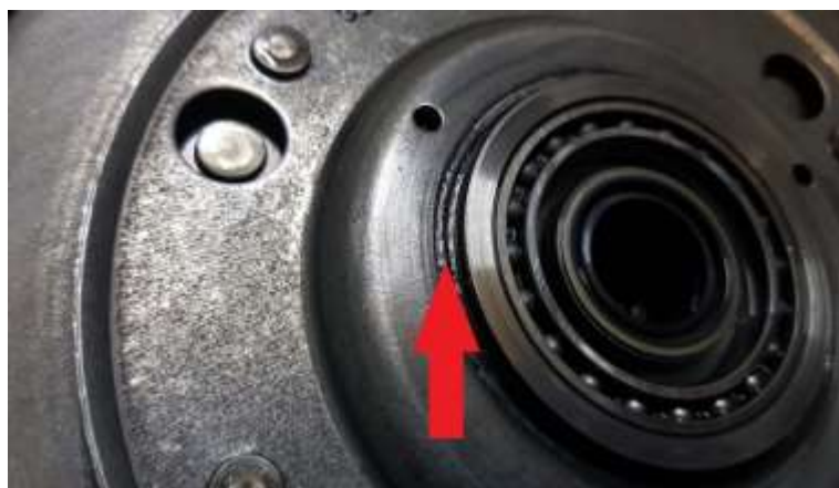
Fig. 6. - Torque converter hub of Belarusian Autoworks car with signs of wear
