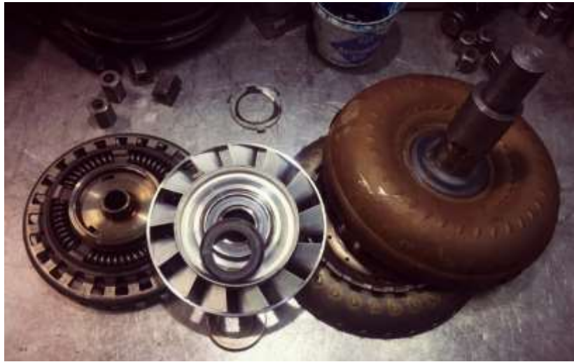
Fig. 4. - Defective torque converter hub
