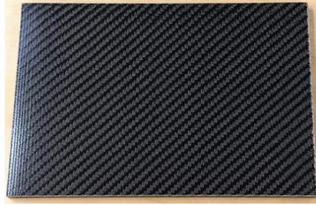
Fig.4. - Laminate 1 (Carbon+Kevlar+M.S.Wire) after manufacturing.
