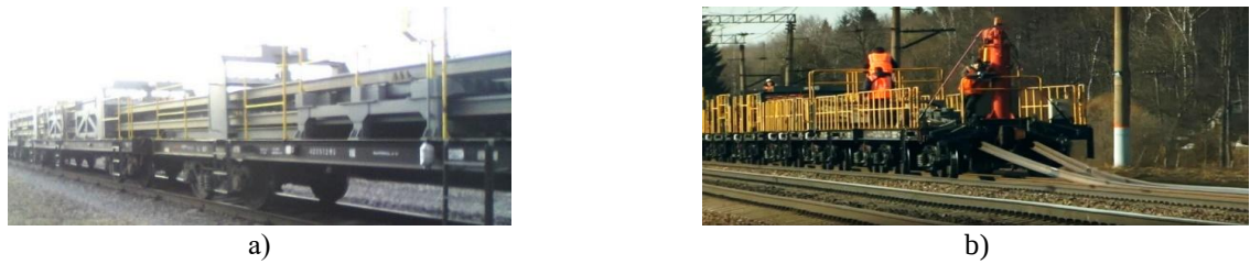
Fig. 1. – Transportation (a) and Laying (b) of Long Welded Rails
