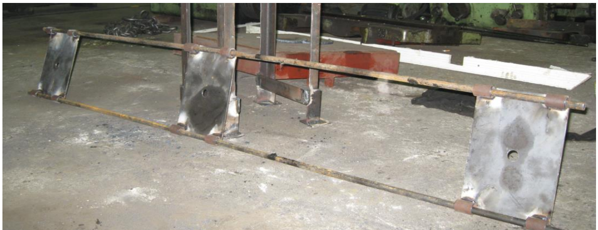
Fig. 17. – An adjustable pickup of the roof bolting
