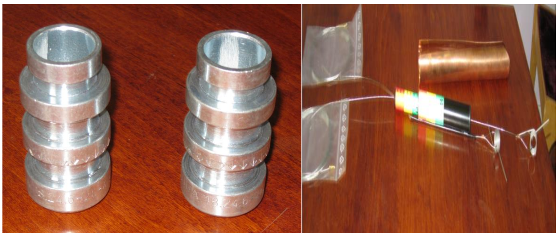
Fig. 5. – Mine pressure regulators and benchmark stations for measuring rock deformations
