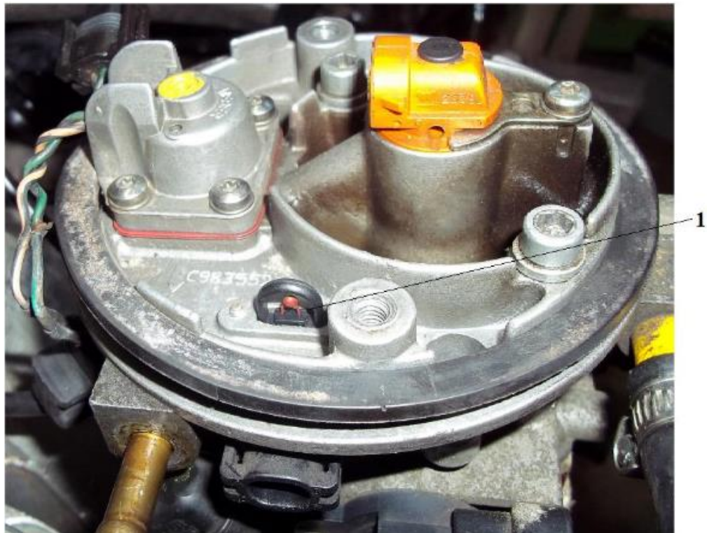
Fig. 4. – Installation location of the intake air temperature sensor, where: 1 – IAT
