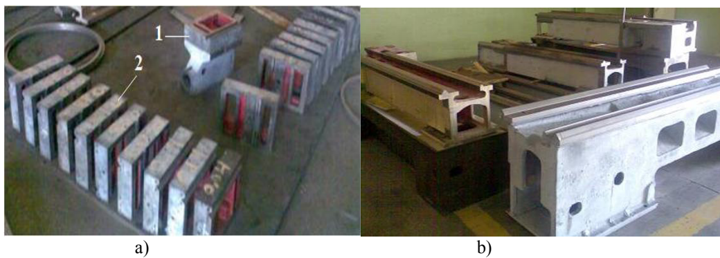
a) tailstock (1) and tailstock plate (2); b) body
