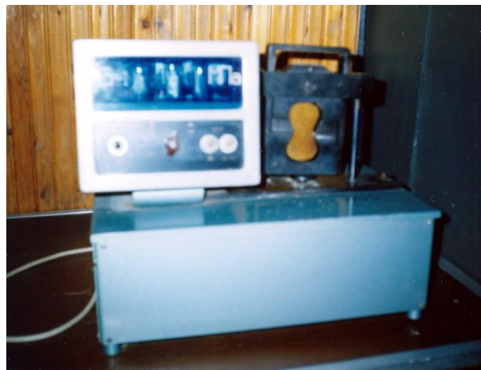
Fig.8 – A sample for determining tensile strength before the testing
