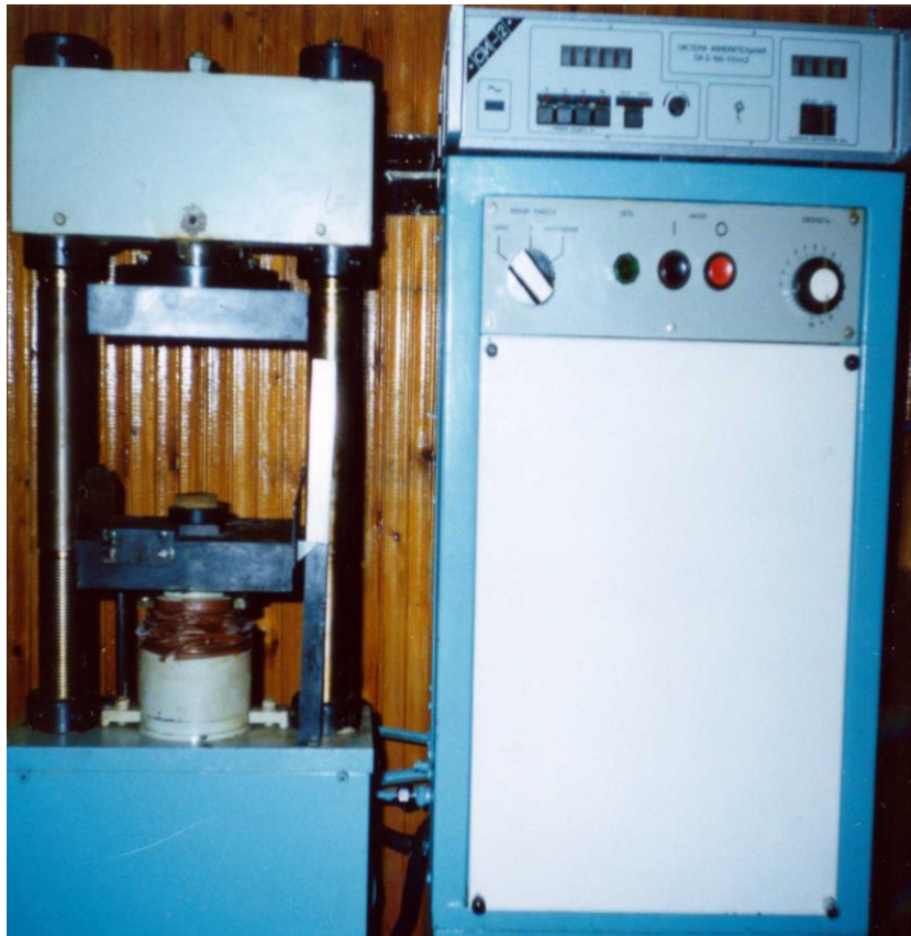
Fig. 9 – A press and a sample for testing compressive strength
