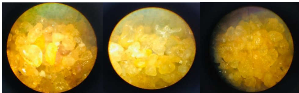
a) 50g of quartz sand + 5g of liquid glass; b) 50 g of quartz sand + 5 g of liquid glass + 5 g of clay; c) 50g quartz sand + 5g liquid glass + 10g clay
