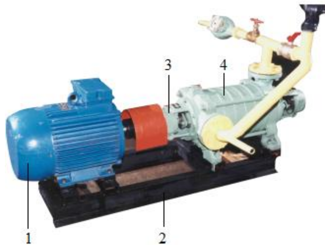
1 – electric motor; 2 – base; 3 – clutch; 4 - pump
