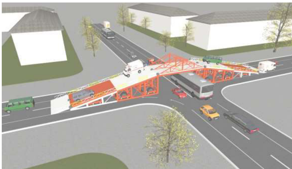
Fig.1 - Mobile road overpass
