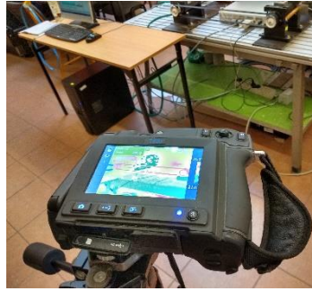
Fig. 1. - A set for testing heat concentration in a flexible connection drive with a NE22 flat belt
