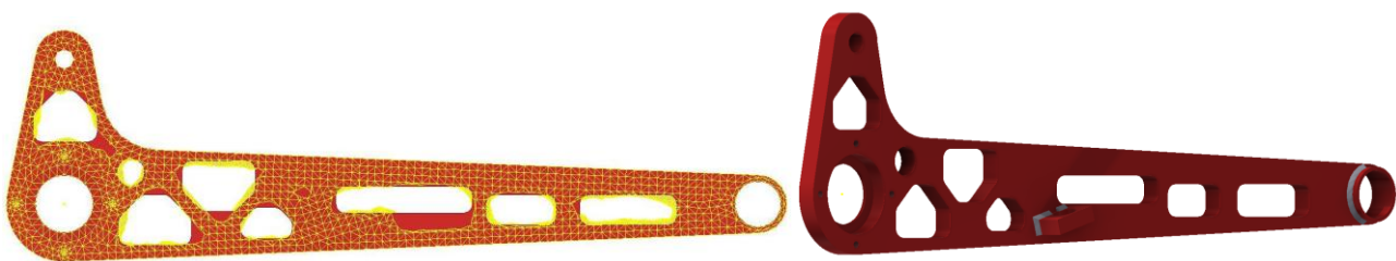
Fig. 7. – Proposed frame geometry after the topological optimization process reducing 30% of the material in the least stressed areas
