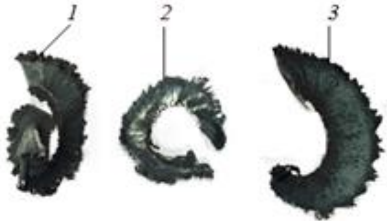
Fig.1. - Photographs of shavings obtained during processing of steel 30HGSA
