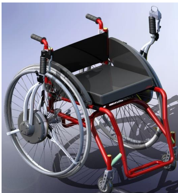
Fig. 8. – Wheelchair lever drive system
