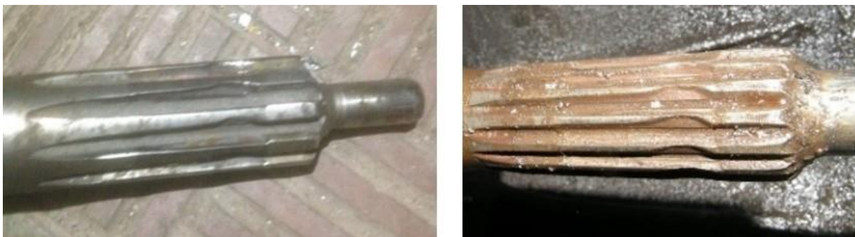
Fig.3. – Wear of spline shafts
