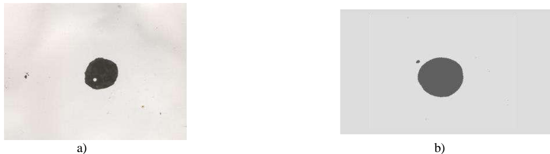
Fig. 3. – Globular nonmetallic inclusions in steels of grades 110G13L (a) and 40X (b), deoxidized by FSA
