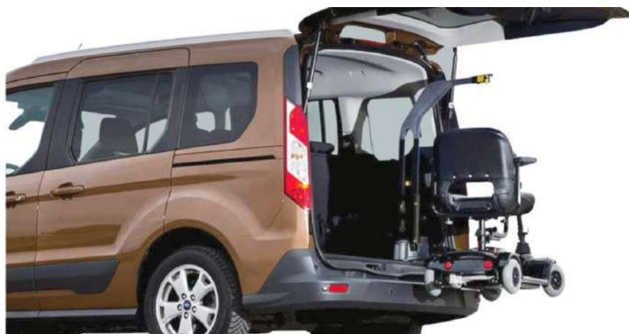
Fig. 5. - BraunAbility wheelchair car lift [10]
