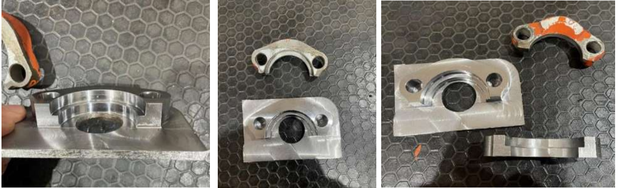
Fig. 11. - The result of processing the product on a milling machine
