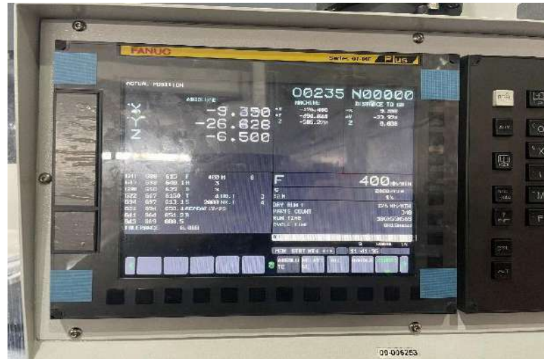
Fig. 2. - The main Fanuc unit for controlling the Akira Seiki milling machine
