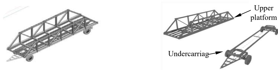
Fig. 1 – Three-dimensional model of a modular overpass
