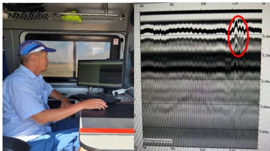
Fig. 4. - Radargram with an anomaly of pavement defects
