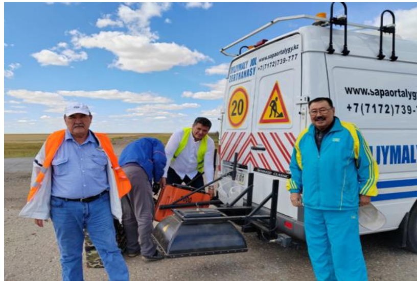
Fig.3. - Mobile road diagnostic laboratory with installed Oko-2 ground penetrating radars, with AB-400R and AB-1000R antenna units
