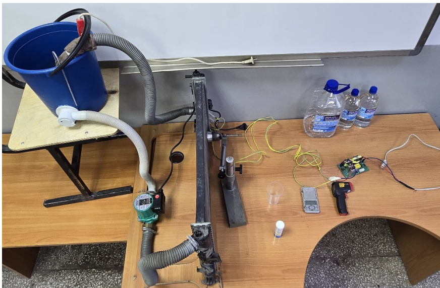
Fig. 3 – Assembled setup for radiator cleaning
