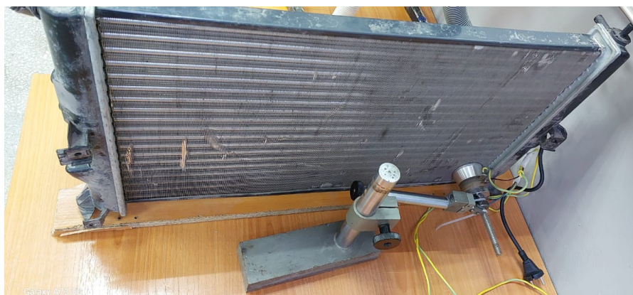
Fig. 4 – Installation of the ultrasonic emitter on the radiator
