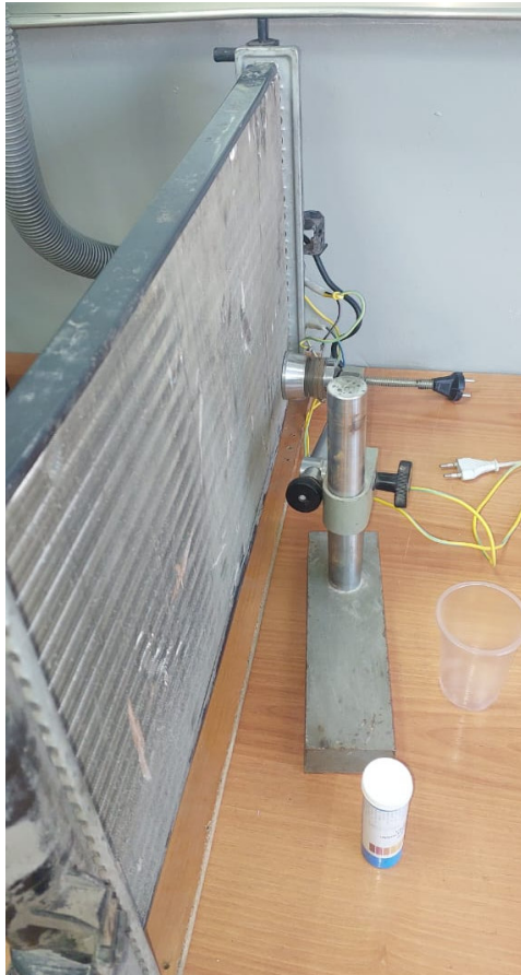
Fig. 5 – Ultrasonic impact on the radiator
