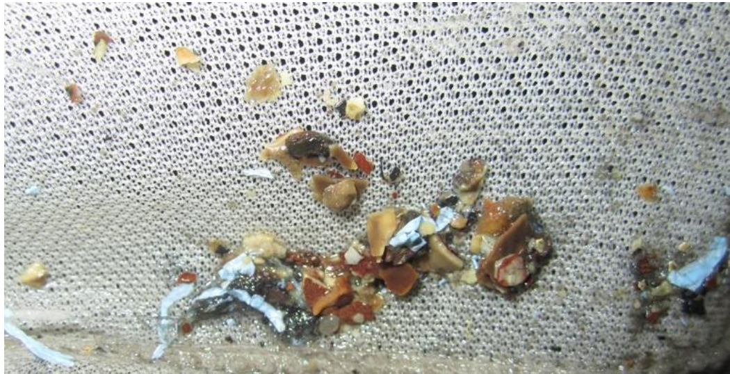
Fig. 3. – Washed scale after exposure to ultrasound
