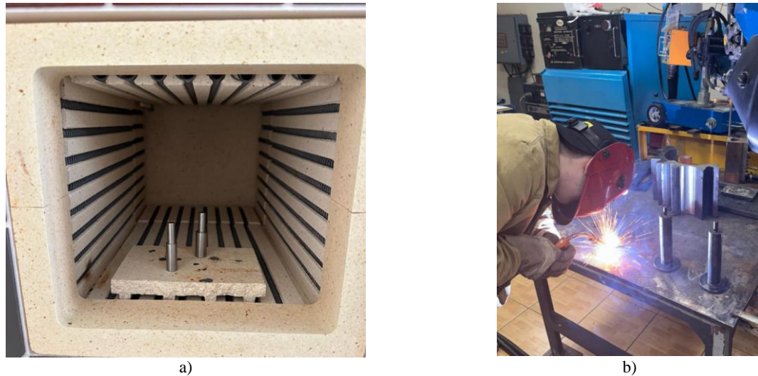
Fig. 3. - Heat treatment in the SNOL 3/1100 muffle furnace (a) and the tool assembly process (b)
