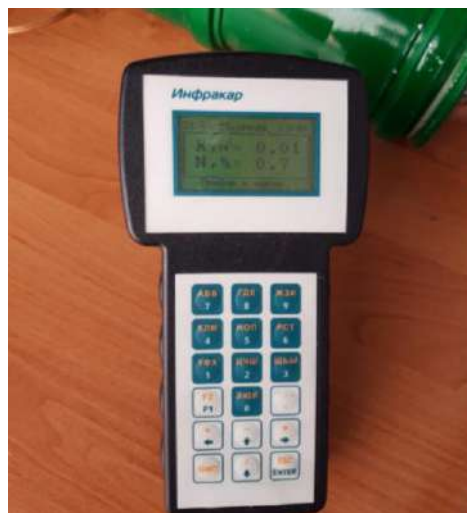
Fig. 5. – Readings of the smoke meter "INFRAKAR-D 1-3.01"
