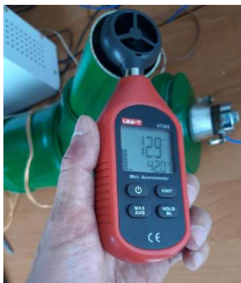
Fig. 8. – Process of measuring exhaust gas velocity
