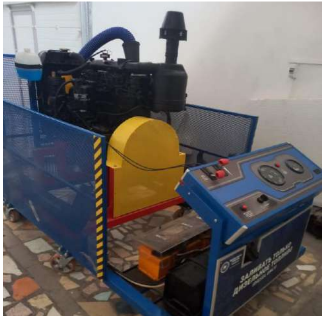
Fig. 1. – Laboratory diesel internal combustion engine "D245"
