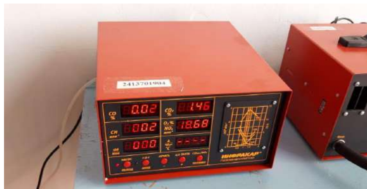
Fig. 4. – Indications of the automobile 4-component gas analyzer "Infrakar M-1.01"
