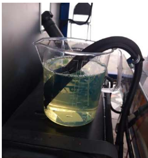
Fig. 7. – Process of measuring fuel consumption
