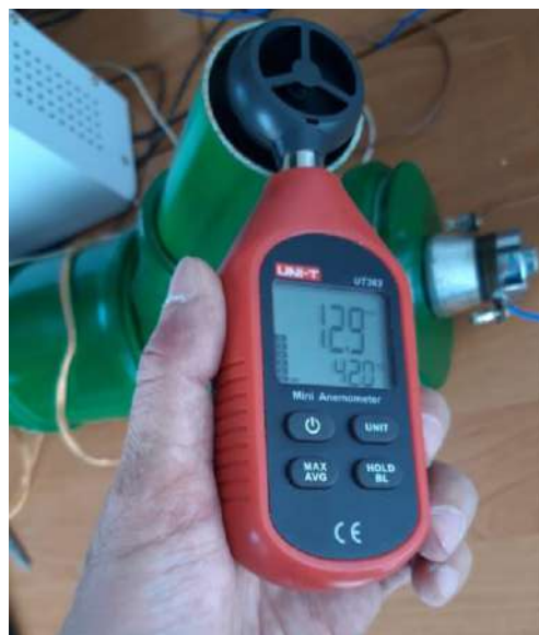
Fig. 8. – Process of measuring exhaust gas velocity
