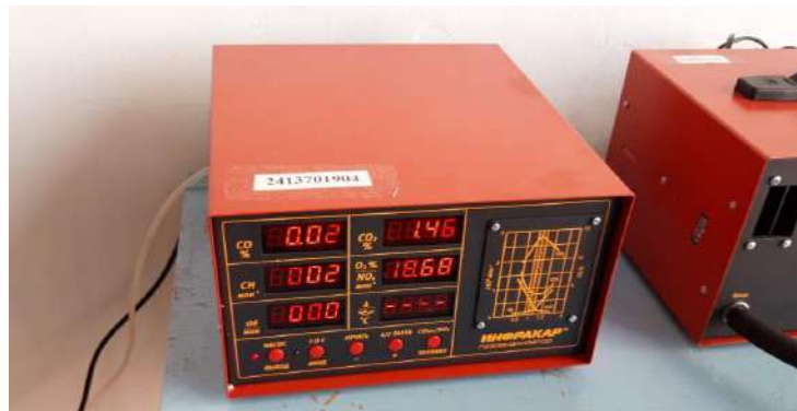
Fig. 4. – Indications of the automobile 4-component gas analyzer "Инфрак M-1.01"
