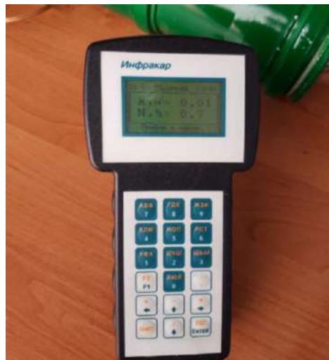
Fig. 5. – Readings of the smoke meter "ИНФРАКАР-D 1-3.01"
