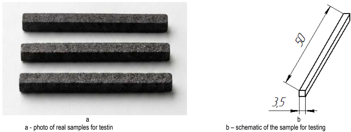
Fig. 2 – Samples for investigating the coefficient of linear thermal expansion
