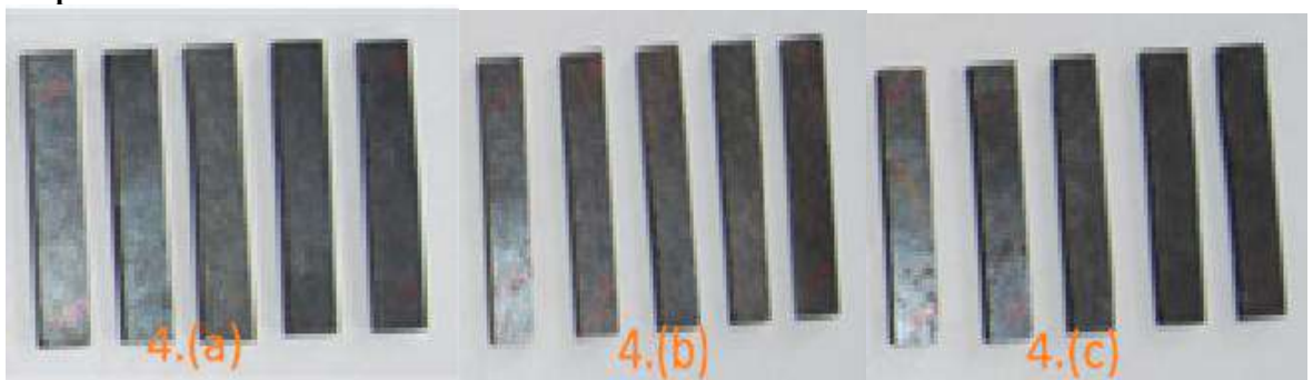
Fig. 4. - The impact test specimen of (a) 0.5 wt % addition of carbon nanoparticle composites (b) 1.0 wt % addition of carbon nanoparticle composites (c) 1.5 wt % addition of carbon nanoparticle composites
