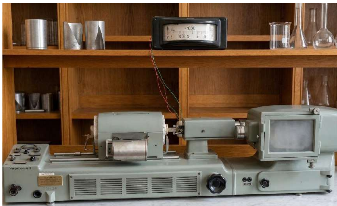
Fig. 1 – Photo of the Chevenard dilatometer setup
