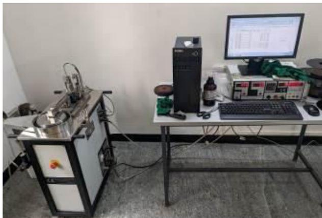
Fig.5. - Pin on disc wear test rig
