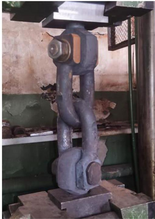
Рис. 8. – Installed mounting blocks on the UMM-100 machine
