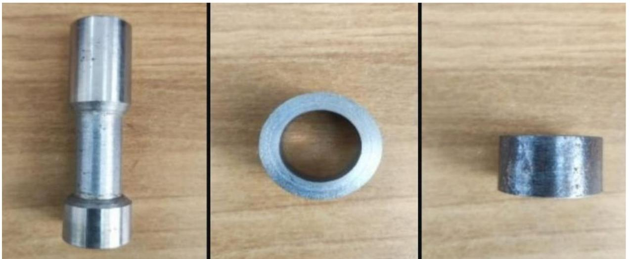
**Fig. 1.** - Punch and press prepared for briquette production
