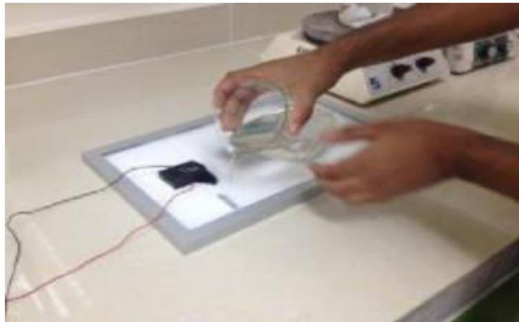
**Fig. 7.** - Melted PCM pouring on the rear part of PV [39]
