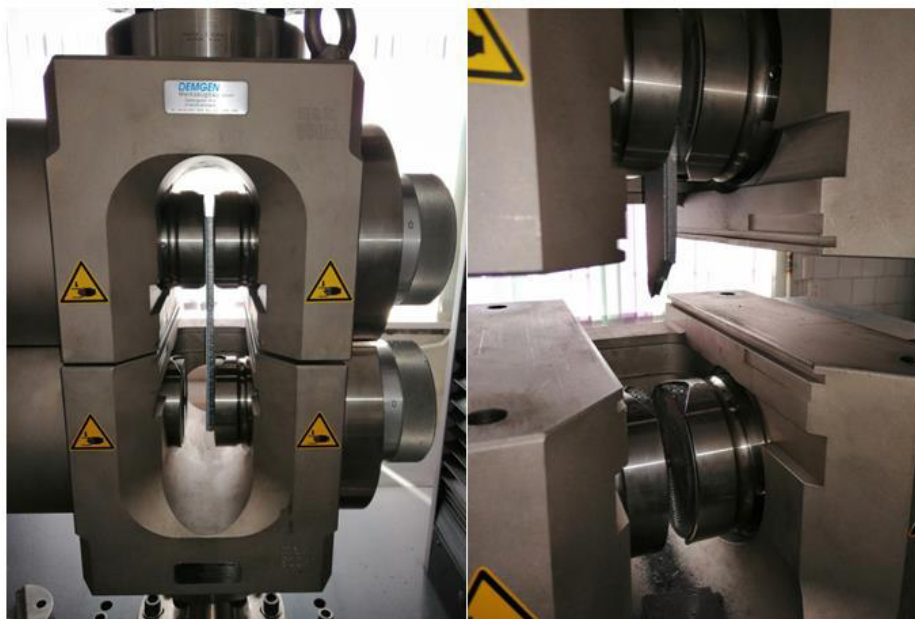
Fig. 7 – Machine for break testing the samples (MTS Company)
