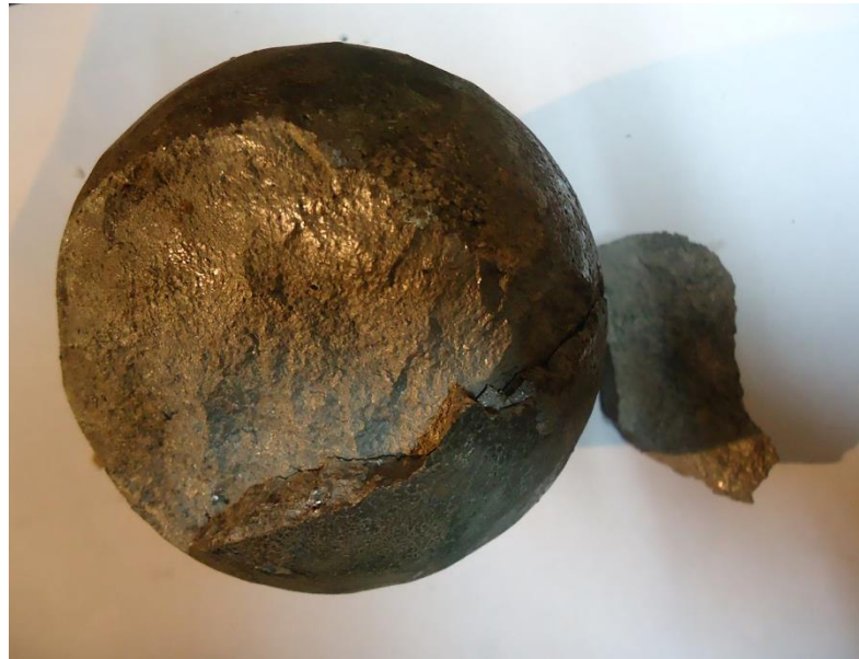
Fig.3. - Cracks on the ball surface, leading to splitting and peeling of the surface
