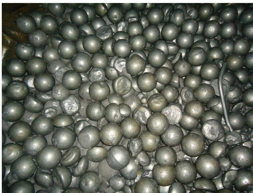
Fig.1. - The piercing of balls \varnothing 100 mm (about 75% of the spherical surface) in an lattice mill ball is 3.2 \times 3.1 , n = 18 rpm
