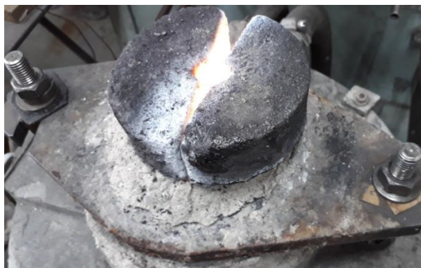
Fig. 6. – Tamman smelting furnace in the process of iron smelting
