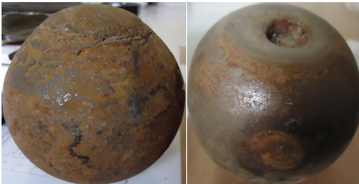
Fig.3. – Rolled steel balls with external defects
