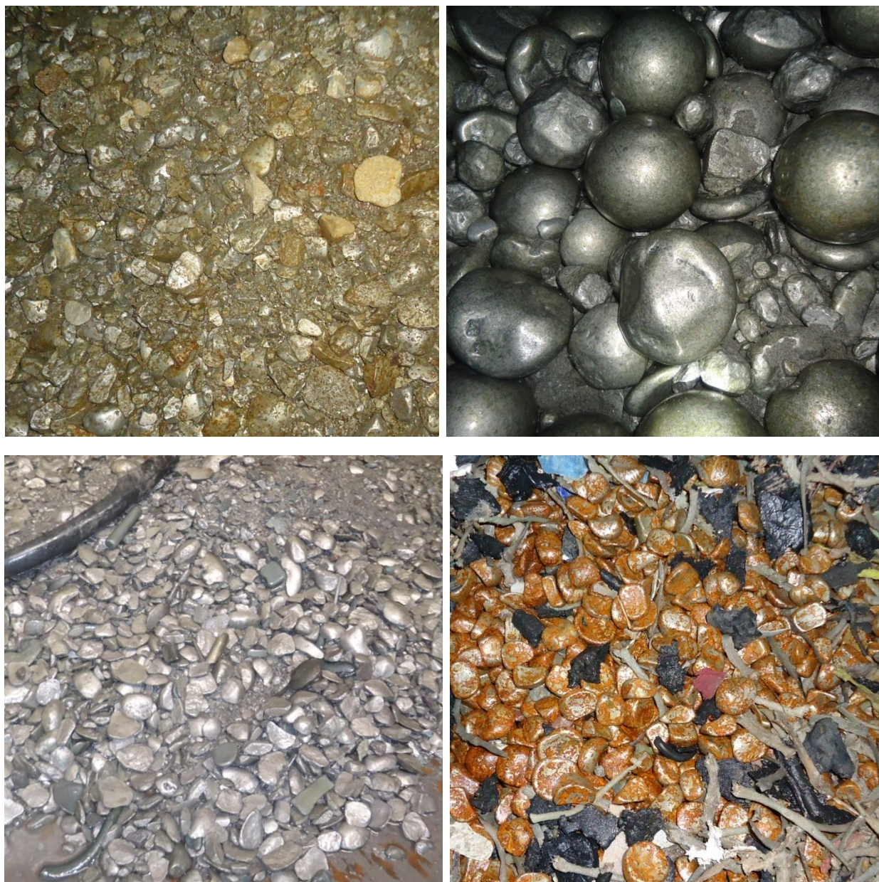
Fig. 4. – Scrap formed in ball mills as a result of grinding balls
