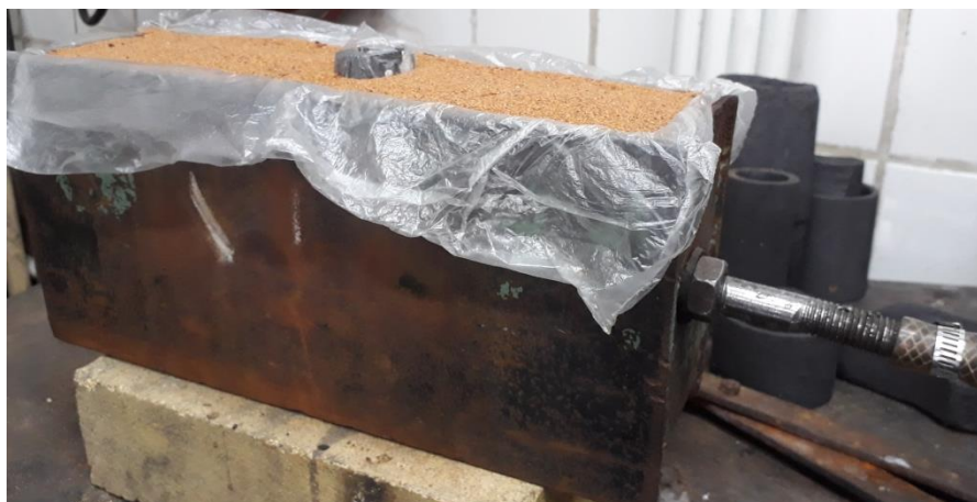
Fig. 8. – Vacuum form, prepared for cast iron casting
