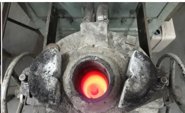
Fig. 6. – Tamman smelting furnace in the process of iron smelting
