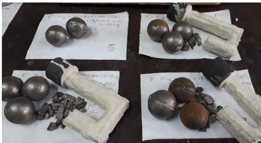
Fig. 7. – Metallic charge and polystyrene foam models prepared for casting samples
