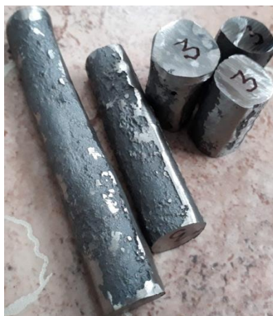
Fig.9. – Modified cast iron cast rods for making samples
