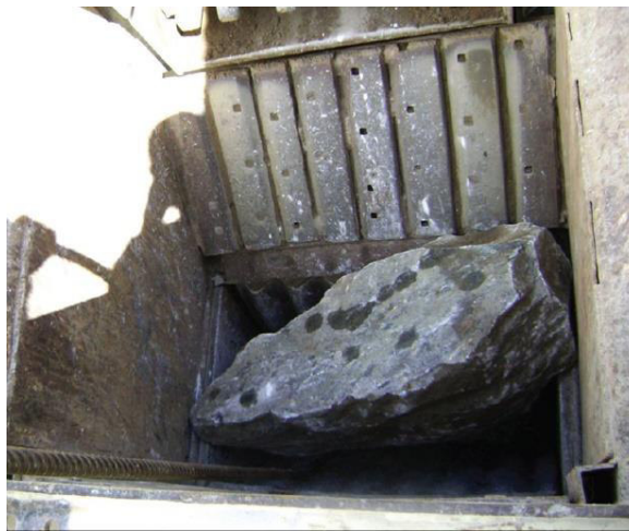
Fig 3. – Oversize at jaw crusher inlet
