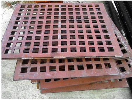
Fig. 1 - Sieve made of Hardox steel
