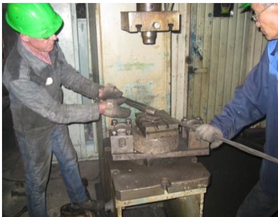
Fig.7. – Twisting the wire rods on the adjacent-spaced machines
