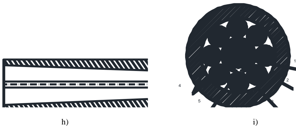
h, i - supporting sleeve profile and its section 1 - central wedge; 2, 3 - outer and inner surfaces of the sleeve clip; 4 - strands of rope; 5 - clamping centering ring
