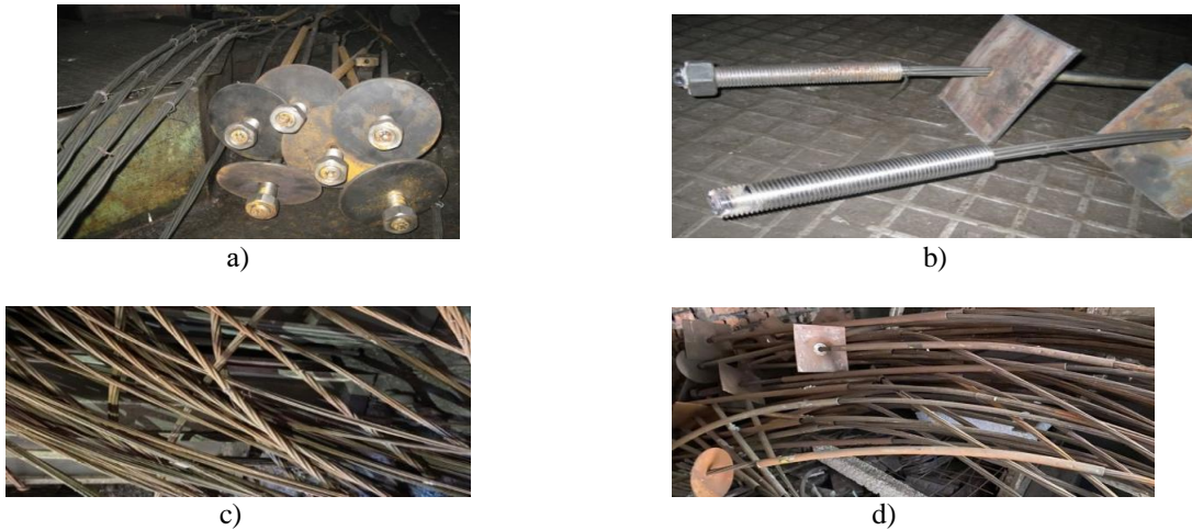
Fig. 11. - Prototypes of rope anchors manufactured at the Karaganda Machine-Building Consortium LLP
