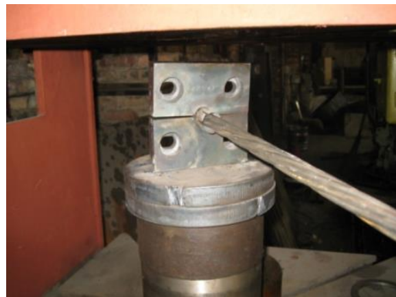
Fig.7. – Twisting the wire rods on the adjacent-spaced machines
