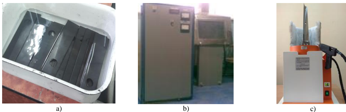
Fig. 3. - Degreasing of hammers with Nefras S2-80/120 (a), polishing in the bath of the EPP-40 unit (b), steam jet device UPS 4.3-geyser (c)
