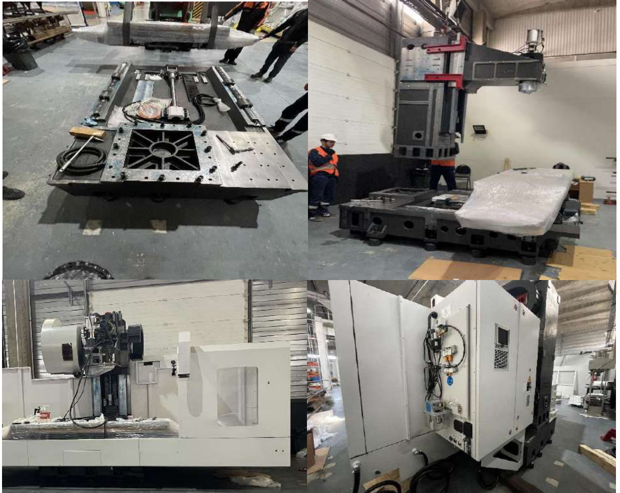
Fig. 1. - Assembling an Akira Seiki machine with Fanuc control software
