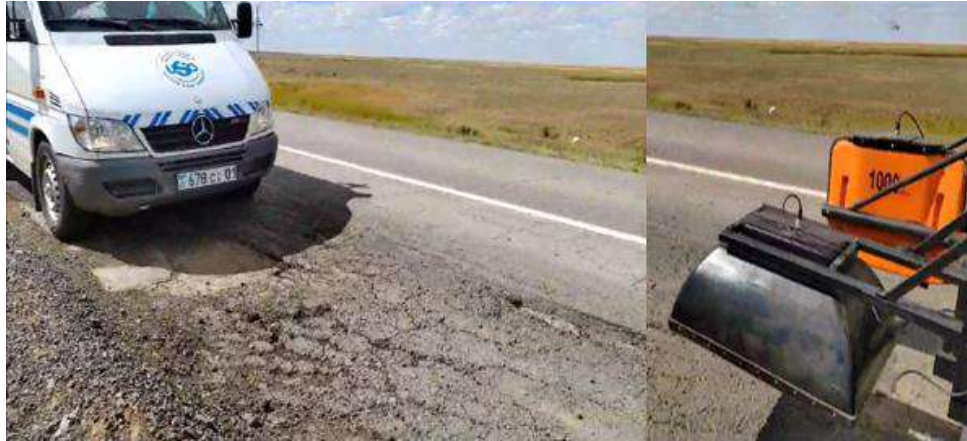
Fig 4. - Surveying with ground penetrating radar anomalies and defects in the road surface of the R-2 “Astana – Korgalzhyn” highway, km 49-51
