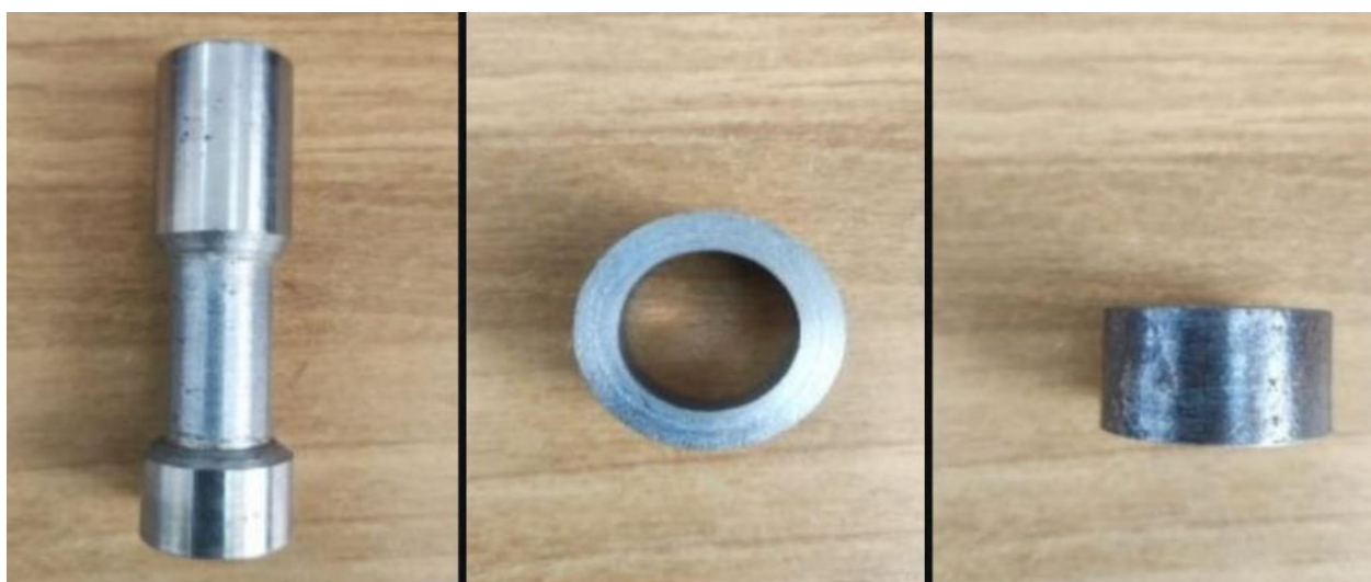
Fig. 1. - Punch and press prepared for briquette production
