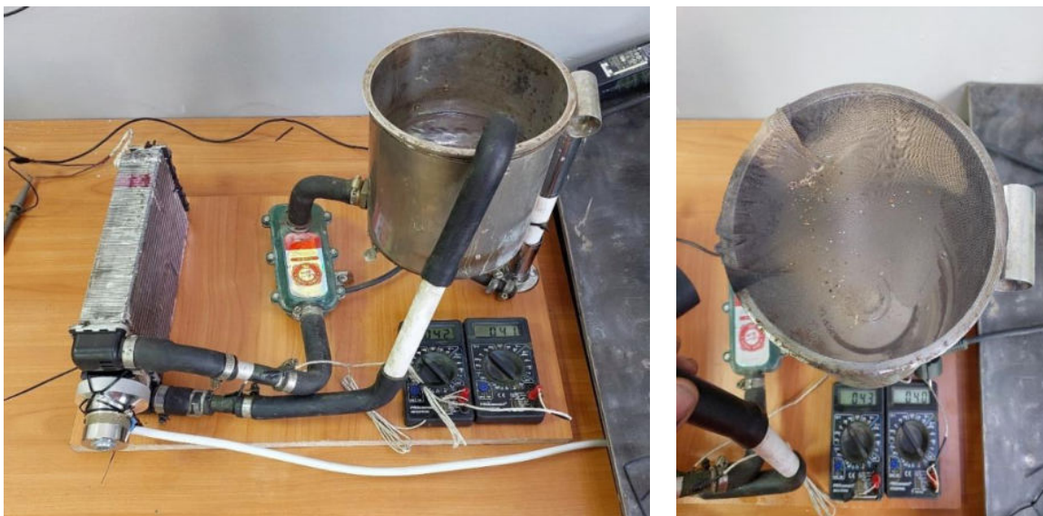
Fig. 2. – Experimental Setup for Ultrasonic Cleaning of Automotive Radiators
