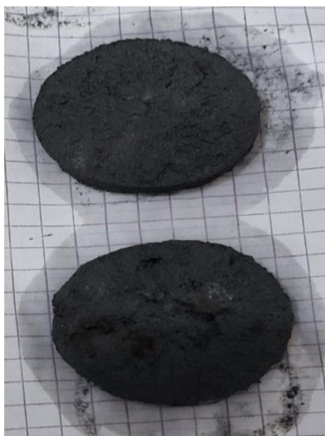
Fig. 3. - Samples of briquettes made from CH15 steel dust chips
