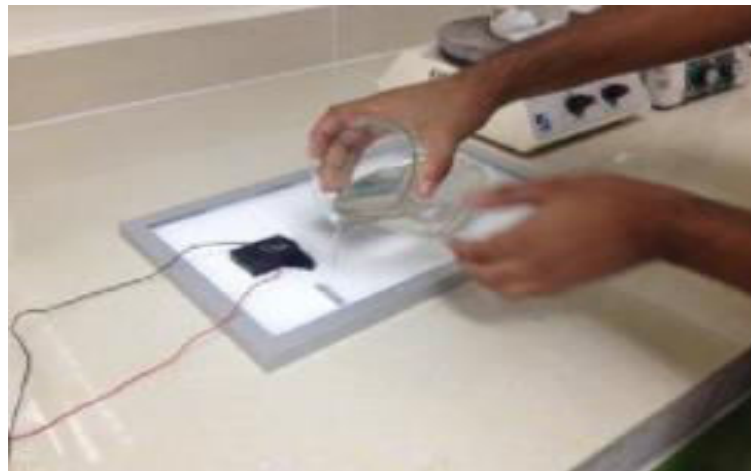
Fig. 7. - Melted PCM pouring on the rear part of PV [39]
