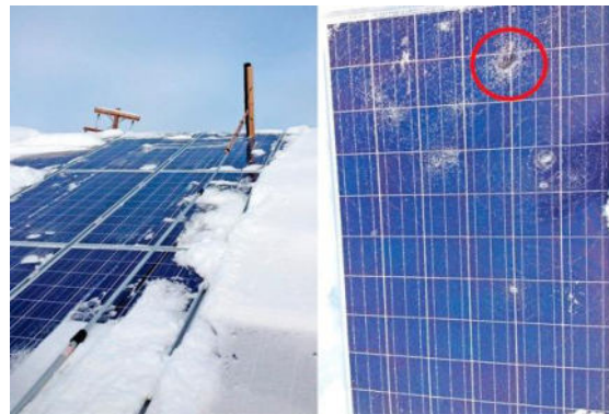
Fig. 13. - The effect of the snow on the model [89]
