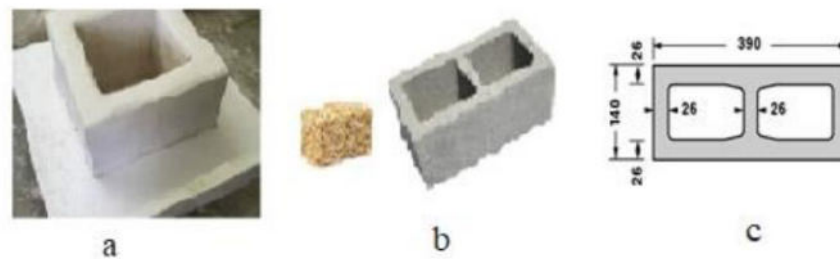
Fig. 1. - a - Test chamber walls b-Straw bell and Brick c- Hollow brick details
