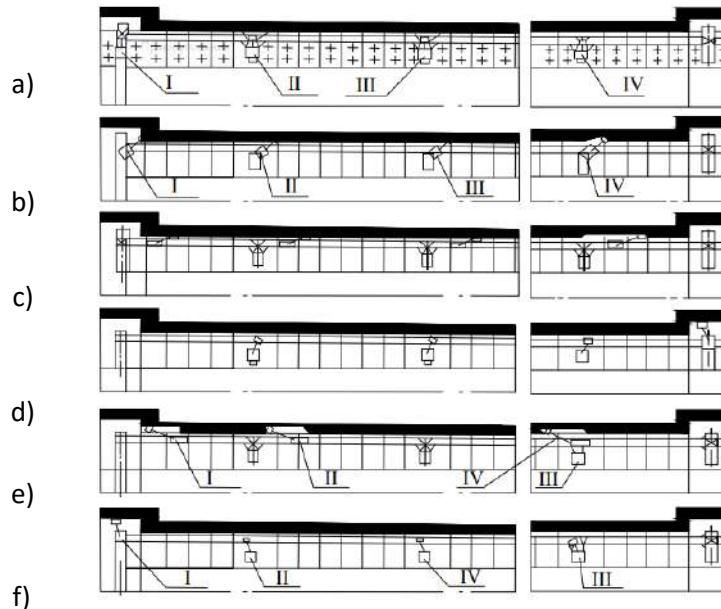
Fig. 4. – Continuous Coal Extraction Technology VMF-5, VMF-6
