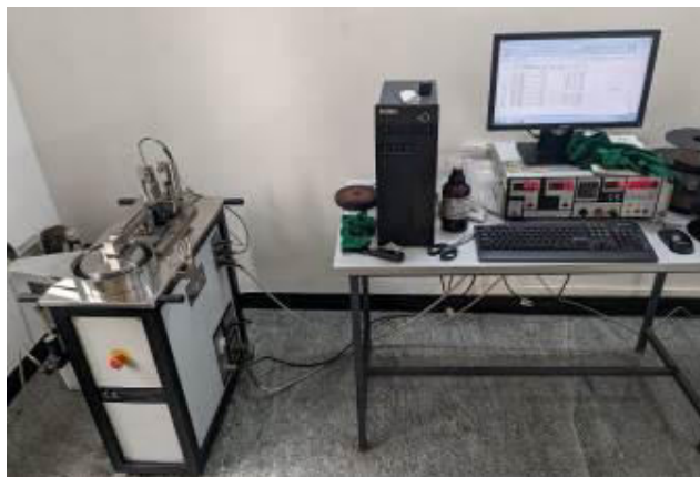
Fig.5. - Pin on disc wear test rig
