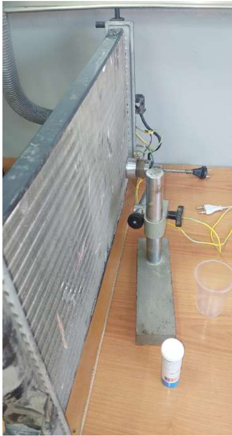
Fig. 5 – Ultrasonic impact on the radiator
