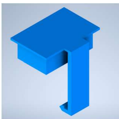
Fig. 3. Model of a snap-on cap used to connect a mesh panel to a post
