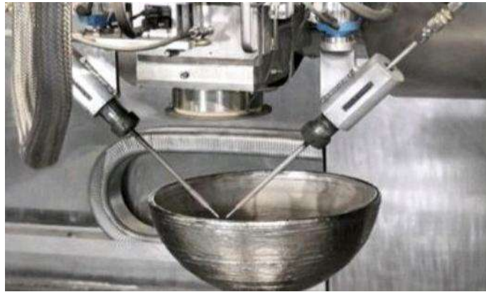
Fig. 3. - Electron beam additive manufacturing using twin wire deposition [44].
