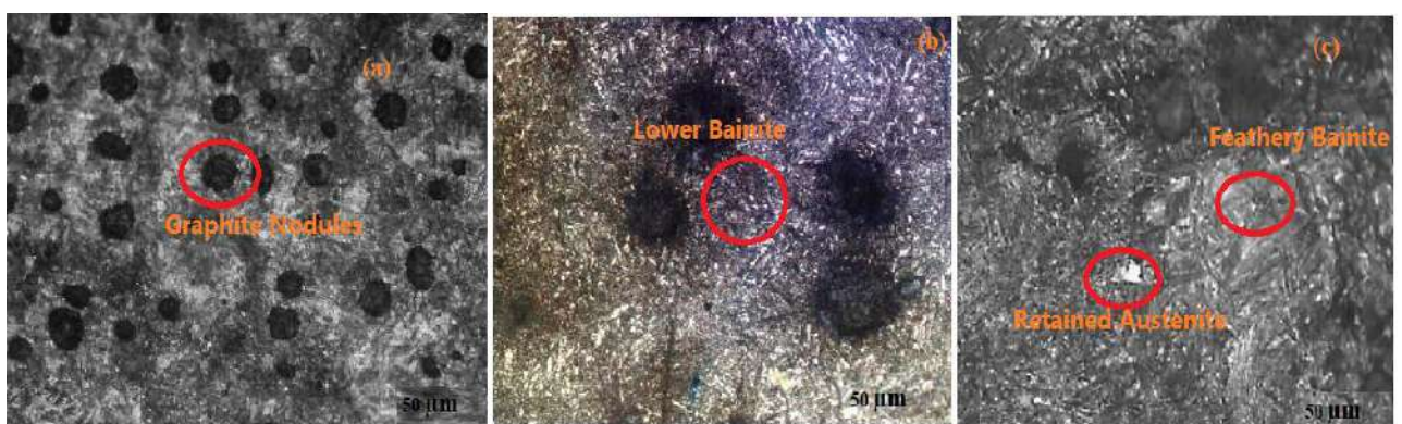
Fig. 3. - (a-c) Micrographs of PMADI 350- Austenizing temperature - 900°C for 120 minutes, Austempering temperature - 350°C for 150 minutes time duration
