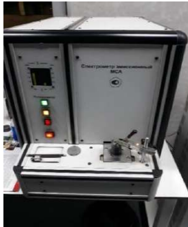
Fig. 3. – Optical-emission spectrometer for chemical composition analysis
