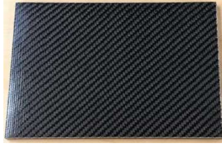
Fig.4. - Laminate 1 (Carbon+Kevlar+M.S.Wire) after manufacturing.
