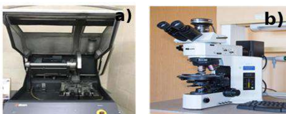
Fig. 5. - Equipment for metallographic research: a) sample preparation device; b) optical microscope
