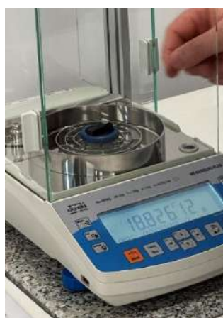
Fig. 4. - Laboratory scales AS 60/220.R2 PLUS Analytical Balance
