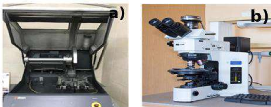
Fig. 5. - Equipment for metallographic research: a) sample preparation device; b) optical microscope
