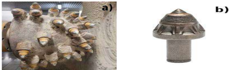
Fig. 1. - The rotating performing body for rock destruction and the wear-resistant coating on the conical geometry mining knife: a) the general view of the rotating performing Body; B) the mining knife with a melt-coated coating.
